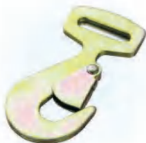
HYFH-073 A=50mm B=160mm C=6mm PULL ≤ 4540KG
