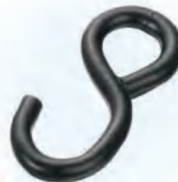
HYSH-060 A=27mm B=110mm C=10mm PULL ≤ 1500KG
